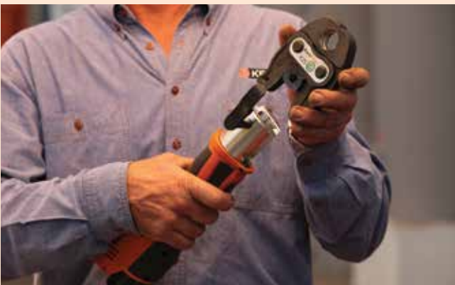
5. Select pressing jaw according to the fitting dimension and insert into the pressing machine. Arrest the locking bolts of the machine. Check the jaws are free from debris and in good working order.
