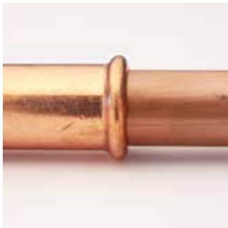
Unpressed fitting - smooth with no indents.
