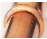
Pressed fitting - no gap between fitting and tube.
