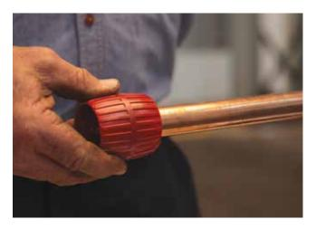
2. Deburr carefully the end of the tube on the inside to minimize turbulence and pressure loss according to the relevant plumbing code and on the outside to avoid damaging the O-ring.
