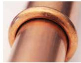
Unpressed fitting - small gap between fitting and tube.
