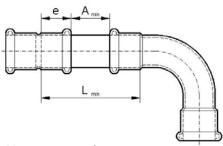
Minimum spacing between two press points. **See table 1.**
