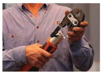
**5.** Select pressing jaw according to the fitting dimension and insert into the pressing machine. Arrest the locking bolts of the machine. Check the jaws are free from debris and in good working order.
